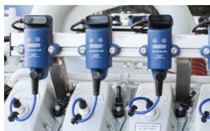
Rail mounting on engine
