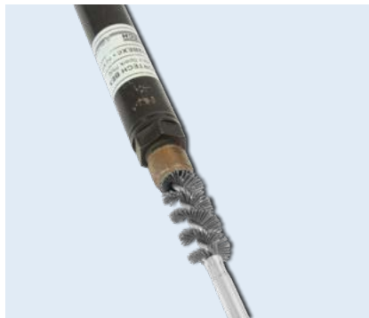
Cleaning of extended barrel spark plug
